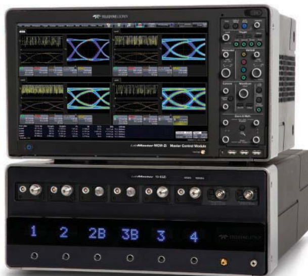
3. The LabMaster 10 Zi oscilloscope systems were recently extended to a measurement range of 100 GHz. [Photo courtesy of Teledyne LeCroy (www.teledyneleeroy.com).]
