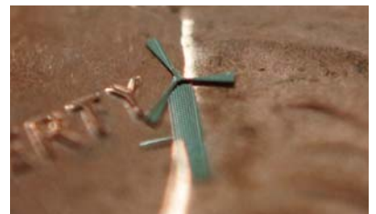
Measuring 1.8 mm at their widest point, micro-windmills developed at UT Arlington could be used to charge portable electronics.
