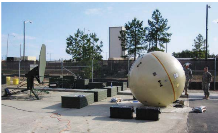
2. Inflatable satcom antennas simplify the use of communications terminals in remote locations. [Photo courtesy of GATR Technologies ( www.gatr.com )]
